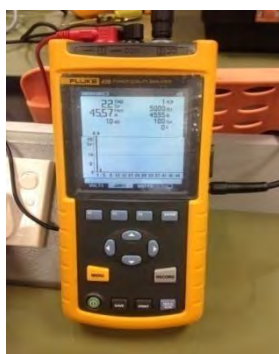
Figure 3.4: Power quality analyzer meter.
