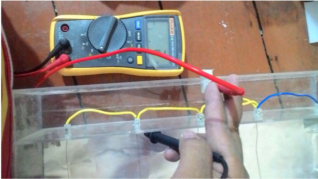
Appendix A: Checking the Connectivity of Cables
