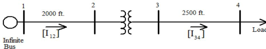
Figure 3.21: IEEE 4-Bus Test Feeder [30]
