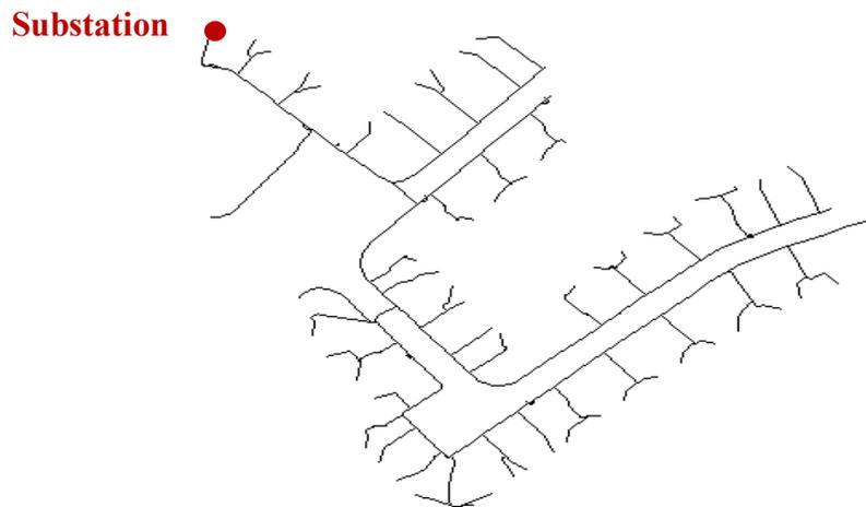
Figure 3.22: One-line Diagram of the European Low Voltage Test Feeder
