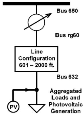
Figure 3.3: The Simplified Node Test Feeder [7]
