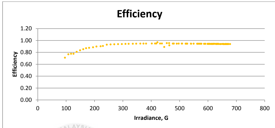
Figure 4.18: Efficiency of 1 : 1.2 inverter to solar panel
