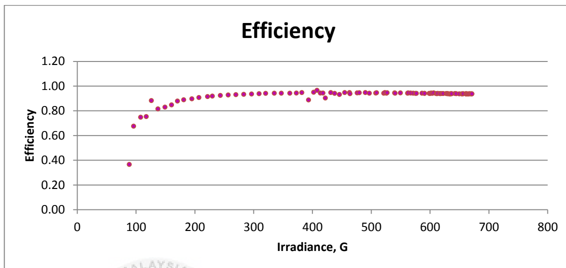
Figure 4.16: Efficiency of 1 : 1.1 inverter to solar panel
