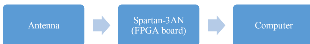
Figure 1.2.2: Signal Processing Flow of Lightning Signals (with FPGA)
