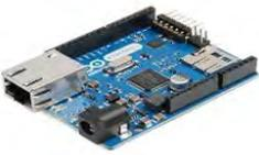
A rectangular blue PCB with a USB Type-B port and an Ethernet port.                                                       | Basically a typical Arduino Uno where the ATMEGA8 chip and the USB fitting are changed for an Ethernet port.                                                                                  |
