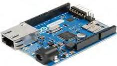
An Arduino Ethernet board, which is a standard Arduino Uno board with an Ethernet port instead of a USB port.           | Basically a typical Arduino Uno where the ATMEGA8 chip and the USB fitting are changed for an Ethernet port.                                                                                  |
