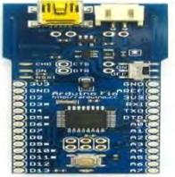
A small, irregularly shaped blue PCB with a USB Type-C port and a yellow LiPo battery connector.                            | An irregular board and is basically an Arduino Mini with an inherent LiPo charger and XBee headers.                                                                                           |
