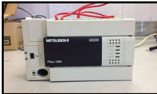
Figure 3.20: FX3u-16M Mitsubishi PLC
