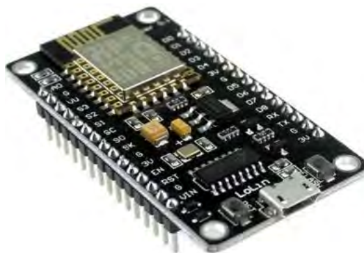
Figure 9: ESP8266-12E NodeMCU development kit V1.0
