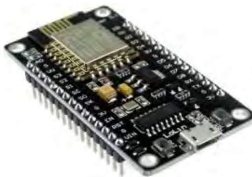
Figure 3: Hardware of ESP8266-12E NodeMCU development board
