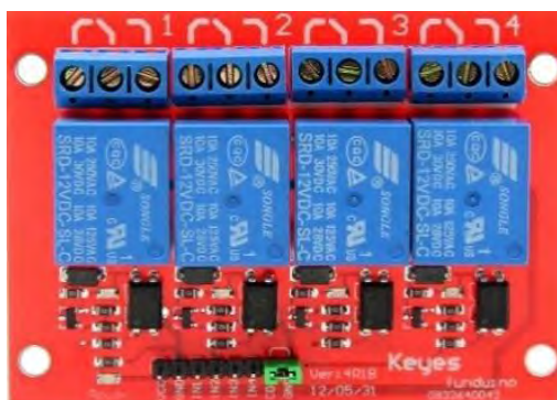
Figure 10: 4-channels 5V relay module
