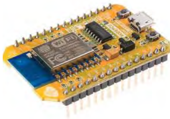
Figure 2: Hardware of ESP8266-12 NodeMCU development board
