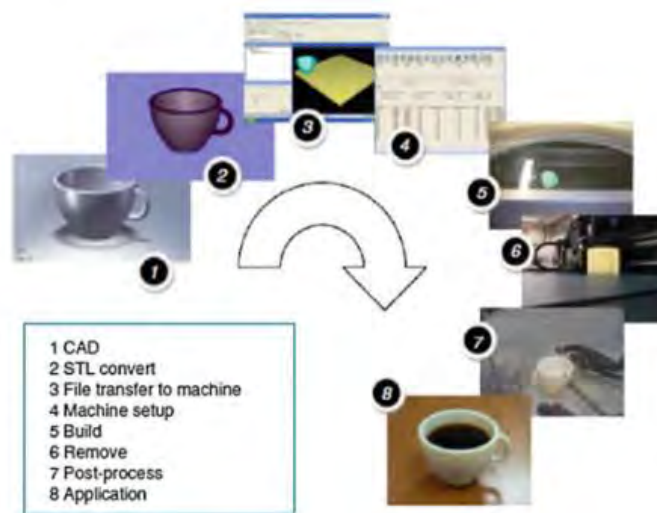
Figure 2.2: Eight Generic AM Processes (Gibson, Rosen, & Stucker, 2010).
