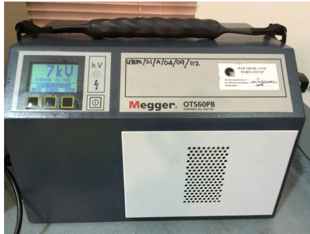
Figure 3.13: Sample Oil inside Megger OTS60PB for BdV Test
