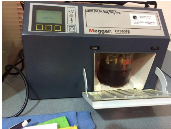
Figure 2.2: Preparation of BdV Test by using Megger OTS60PB
