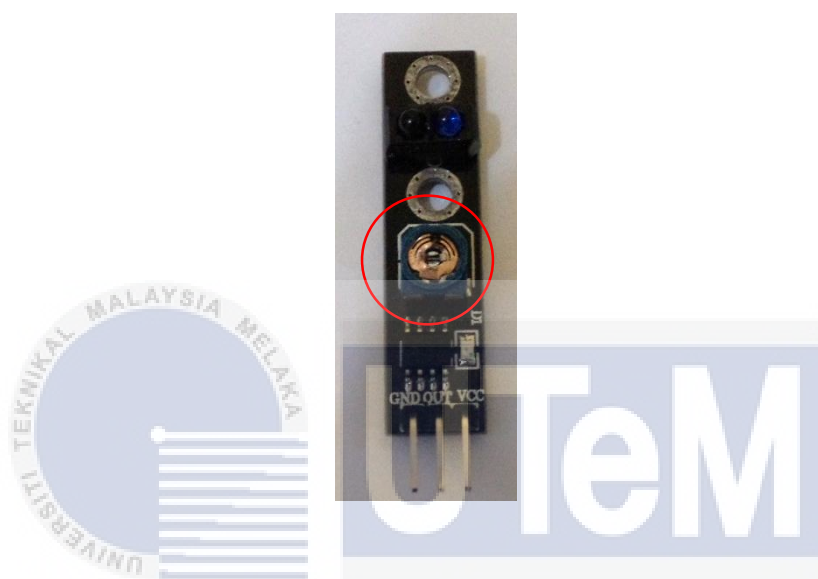
Figure 4.7: The Potentiometer for Distance Control
