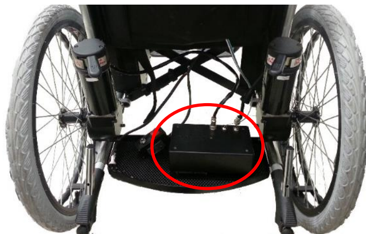
Figure 4.21: Motor driver underneath the wheelchair
