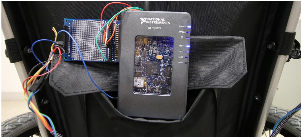
Figure 4.22: Placement of NI myRIO inside the compartment behind the wheelchair
