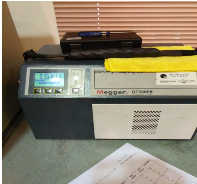
Figure 3.3: Megger breakdown voltage OTS 60PB
