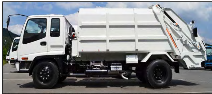
Figure 2.3: Example of Garbage truck installed with a garbage compactor
