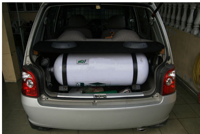
Figure 2.2: Example of CNG Tank Installed in Kancil (Source: Internet Reference , 11/08/09)
