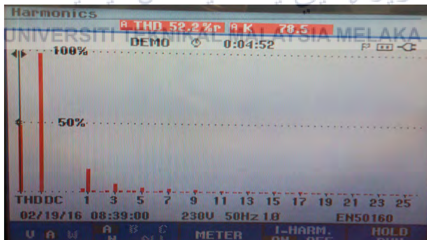
Figure 4.16: Harmonic content in the load current
