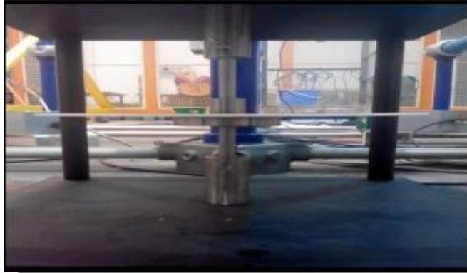
Figure 2.3: actual arrangement of unequal electrode
