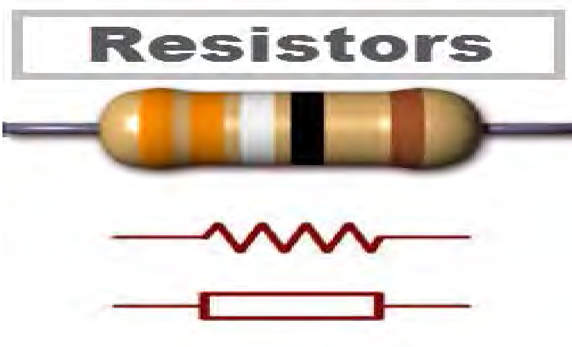
Figure 2.3 typical shape of resistor with its symbol
