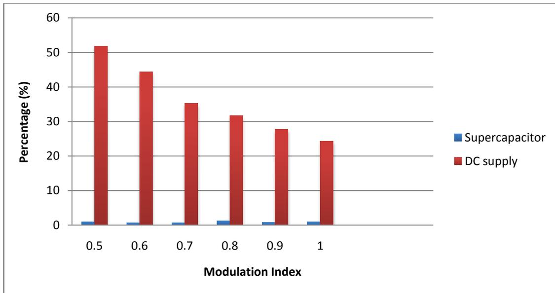
Figure 4.29: Bar Chart of comparison between DC supply and supercapacitor
