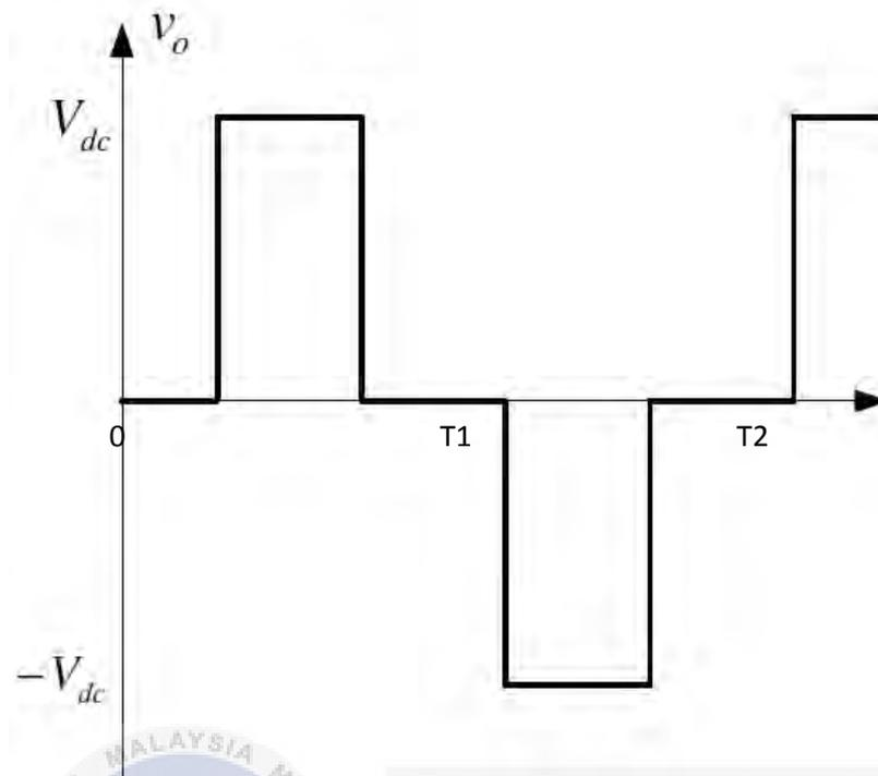
Figure 2.6: Output waveform of basic H-Bridge inverter
