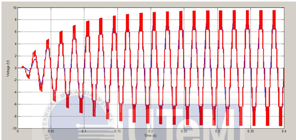
Figure 4.16: Voltage waveform at output seven-level cascaded H-Bridge multilevel inverter which MI= 1.0 using supercapacitor
