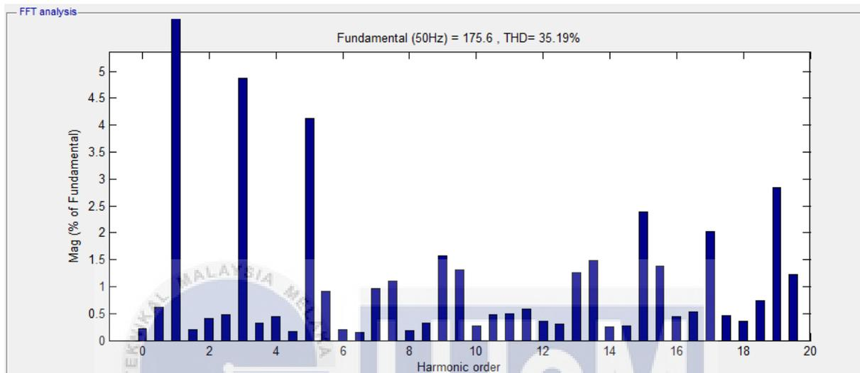
Figure 4.19: Harmonic spectrum for voltage at output seven-level cascaded H-Bridge multilevel inverter which MI = 0.7 using DC Supply
