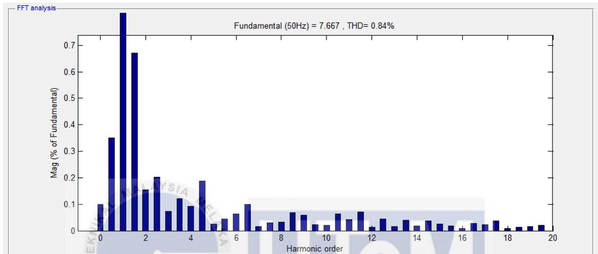
Figure 4.27: Harmonic spectrum for voltage at output seven-level cascaded H-Bridge multilevel inverter which MI = 0.9 using supercapacitor
