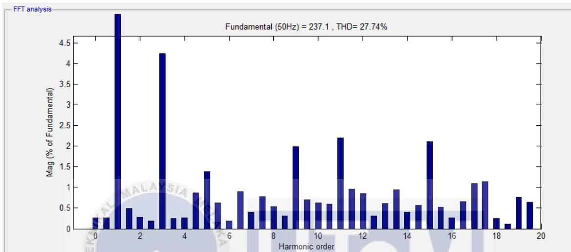
Figure 4.21: Harmonic spectrum for voltage at output seven-level cascaded H-Bridge multilevel inverter which MI = 0.9 using DC Supply
