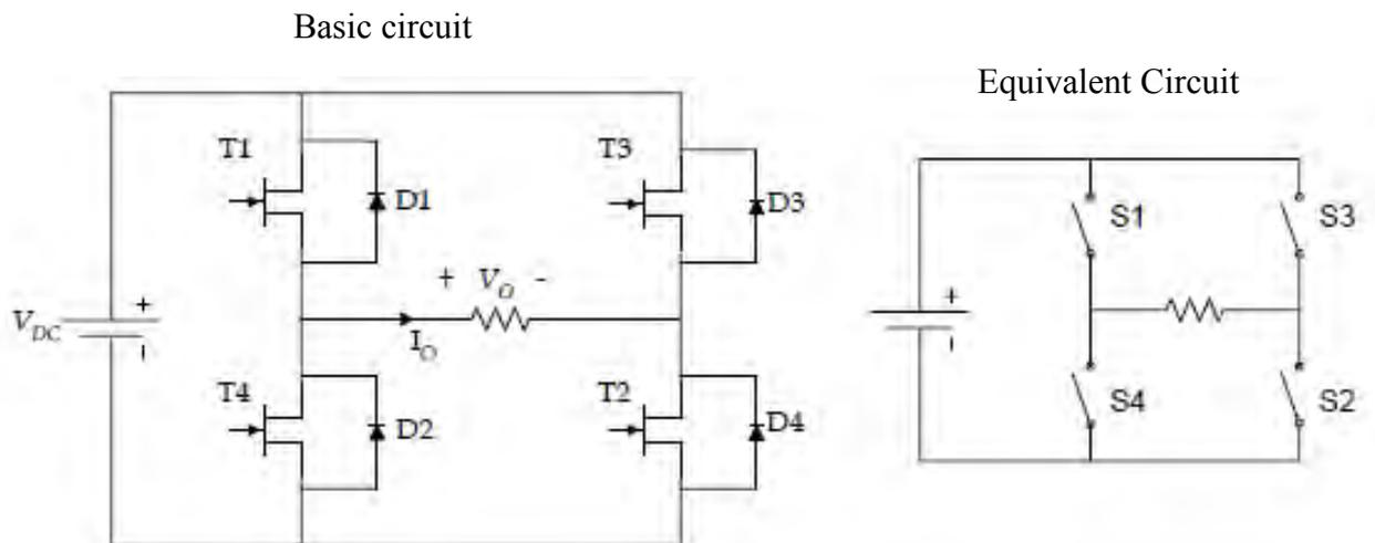
Figure 2.1: Basic circuit and equivalent circuit of inverter
