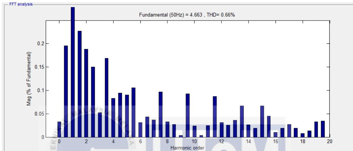
Figure 4.24: Harmonic spectrum for voltage at output seven-level cascaded H-Bridge multilevel inverter which MI = 0.6 using supercapacitor
