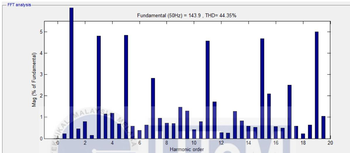
Figure 4.18: Harmonic spectrum for voltage at output seven-level cascaded H-Bridge multilevel inverter which MI = 0.6 using DC Supply
