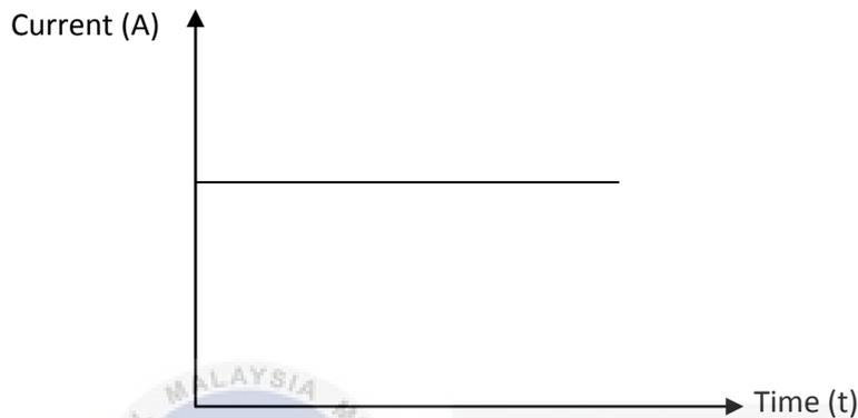
Figure 2.10: Direct current against time graph.
