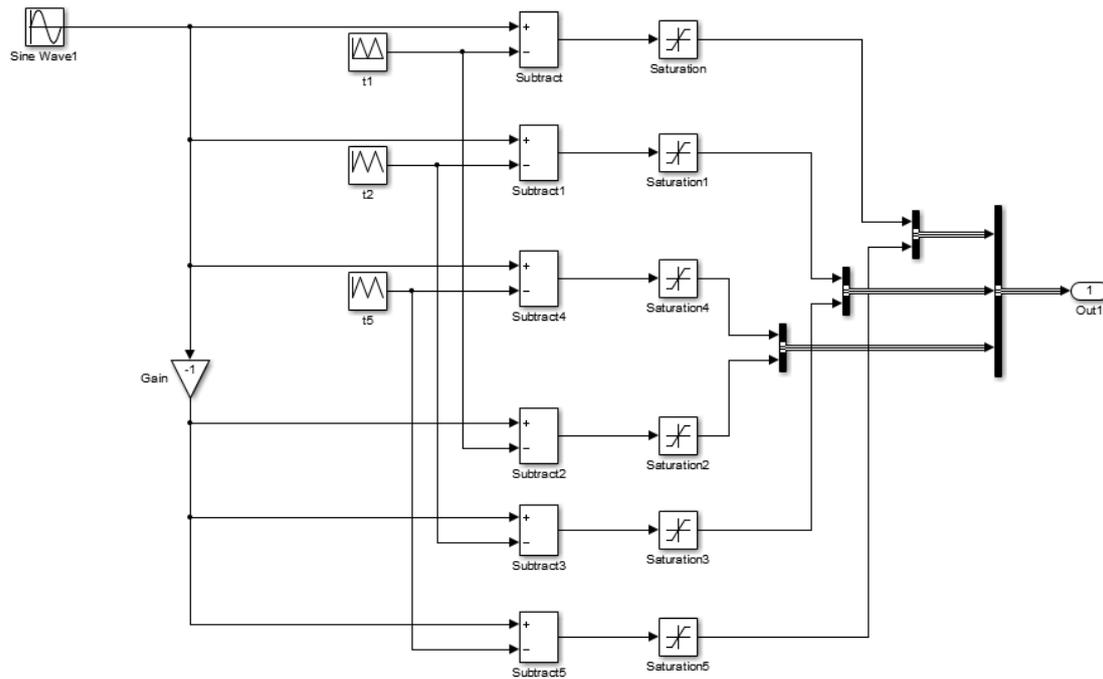
Figure 3.14: Sinusoidal Pulse Width Modulation (SPWM) Controller for seven-level cascaded H-Bridge multilevel inverter.
