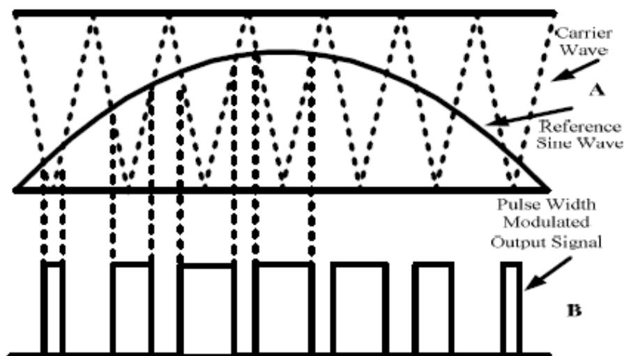
Figure 3.13: Sinusoidal Pulse Width Modulation [21]
