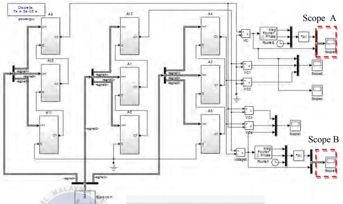
Figure 3.3: Scope for seven-level cascaded H-Bridge multilevel inverter by using MATLAB SIMULINK
