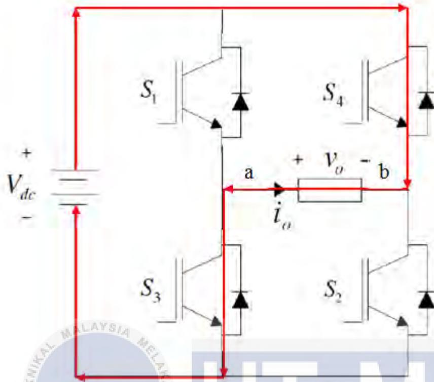
Figure 2.5: Negative cycle of basic H-Bridge inverter
