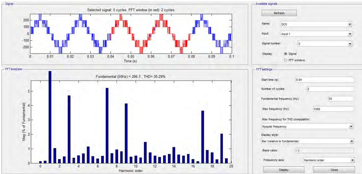
Figure 3.5: Simulation of seven-level cascaded H-Bridge multilevel inverter signal by using Fast Fourier (FFT) Analysis Tool.
