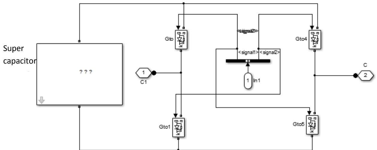
Figure 3.10: Schematic Diagram of Supercapacitor and switching by using MATLAB SIMULINK
