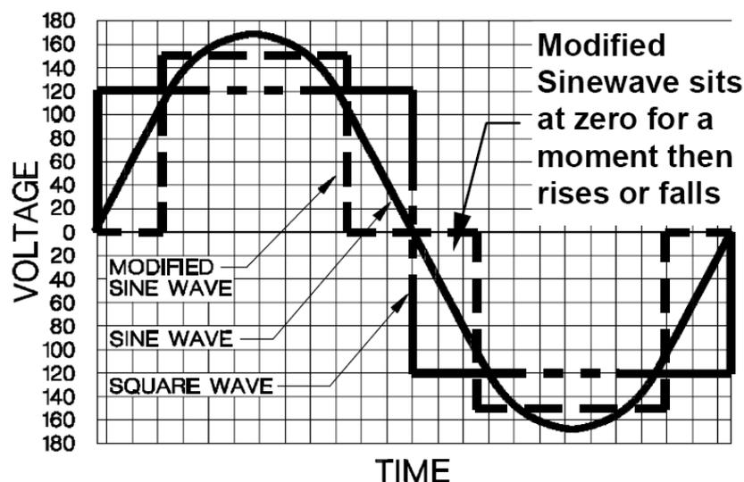
Figure 2.2: Square, Modified and Pure Sine wave
