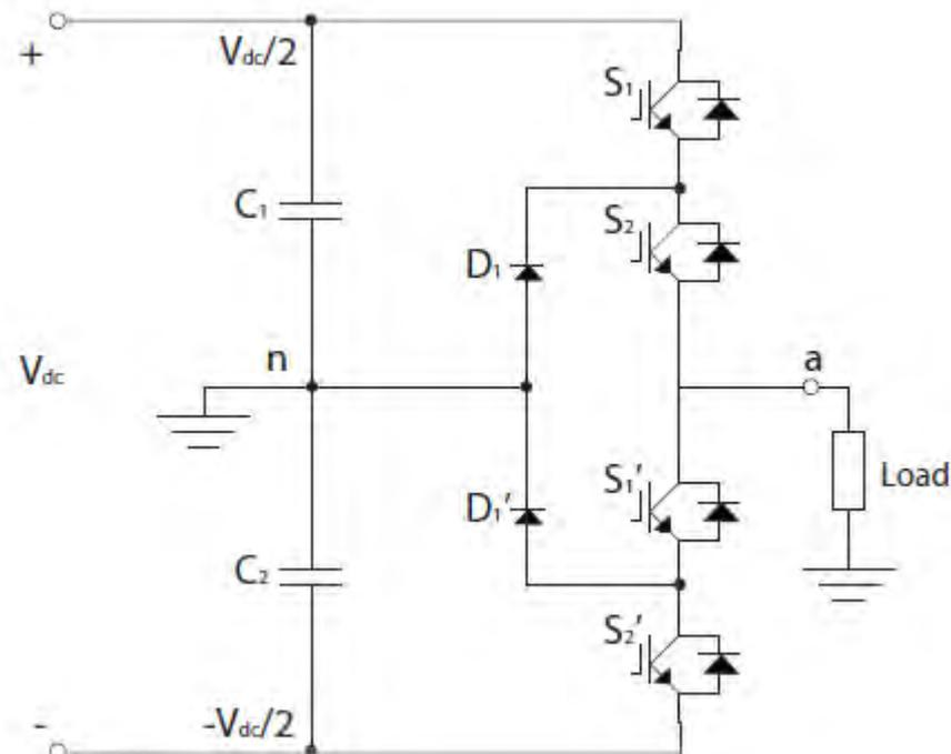
Figure 2.8: One phase leg of a three-level inverter
