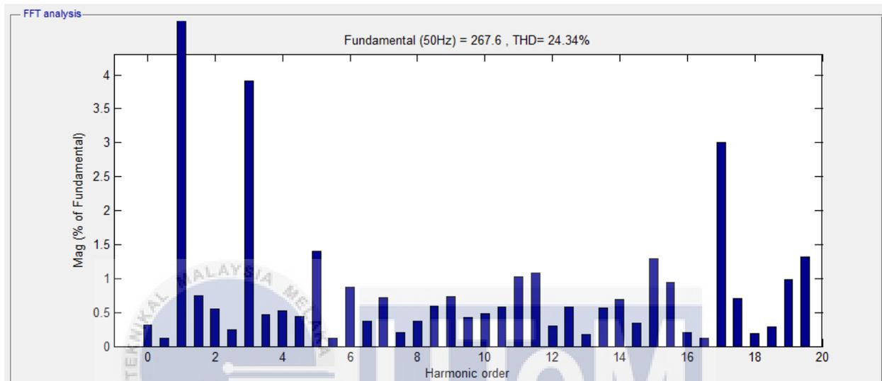
Figure 4.22: Harmonic spectrum for voltage at output seven-level cascaded H-Bridge multilevel inverter which MI = 1.0 using DC Supply
