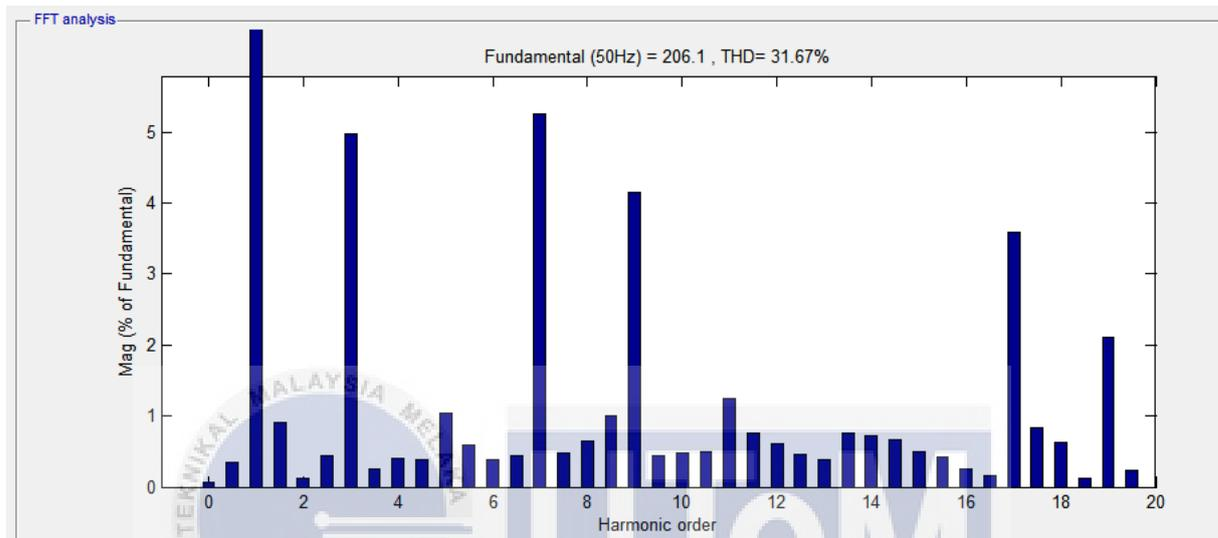
Figure 4.20: Harmonic spectrum for voltage at output seven-level cascaded H-Bridge multilevel inverter which MI = 0.8 using DC Supply
