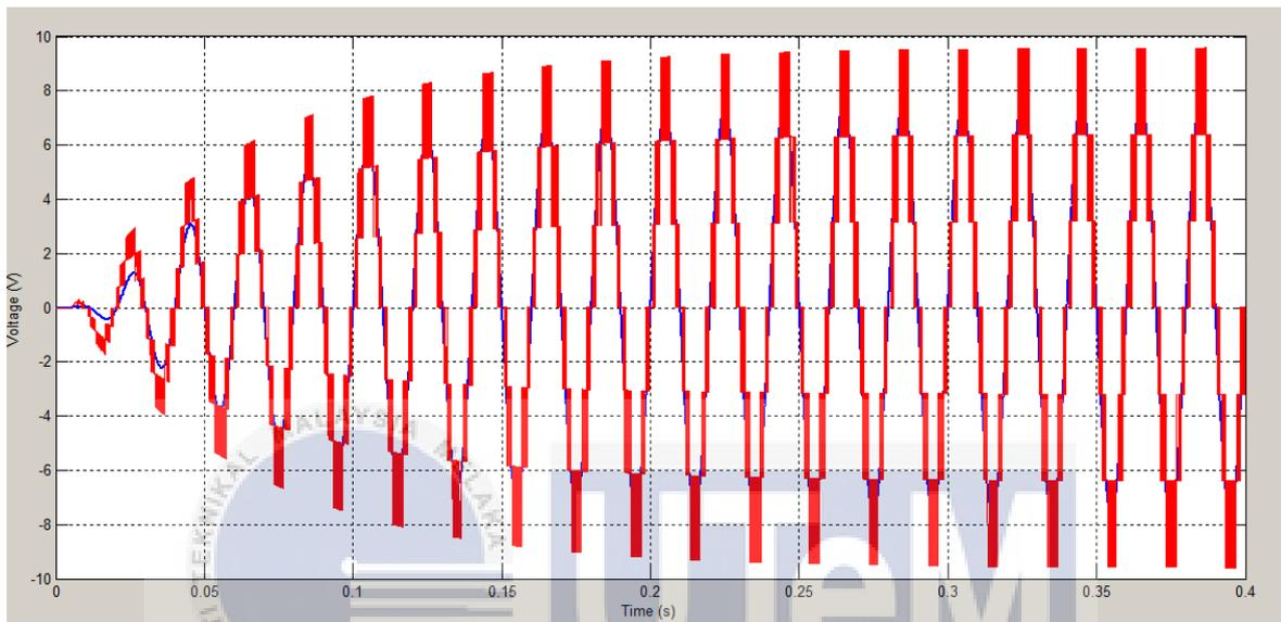
Figure 4.15: Voltage waveform at output seven-level cascaded H-Bridge multilevel inverter which MI= 0.9 using supercapacitor
