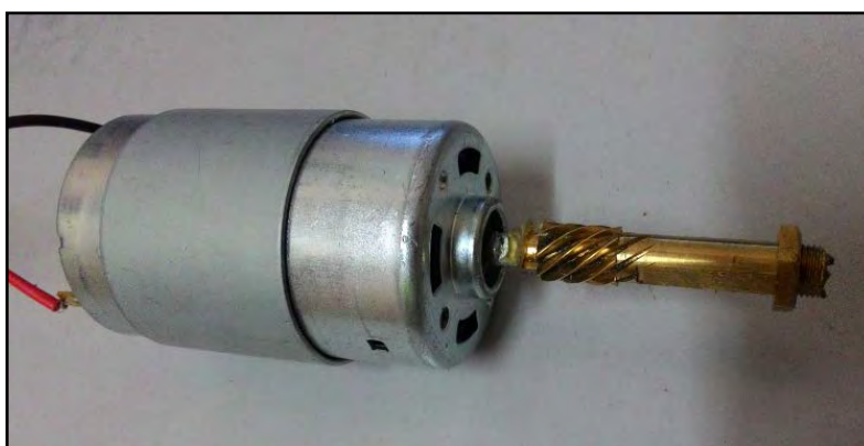
Figure 3.3: DC motor high torque with modified shaft
