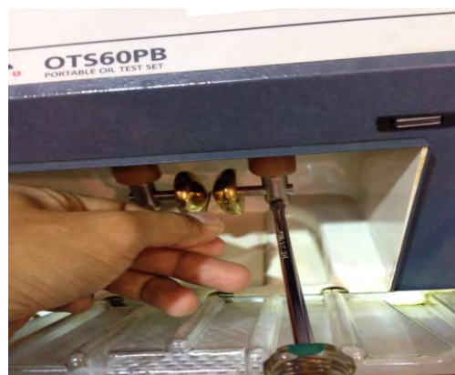
Figure 3.9 : The gap setting between both electrodes
