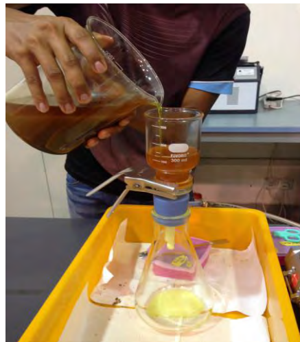
Figure 3.5 : The filtration process by filter paper with the aid of vacuum pump
