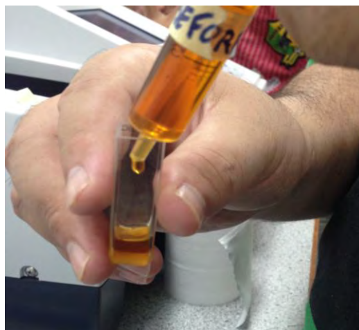
Figure 3.7 : The placement of oil sample into cuvette using syringe
