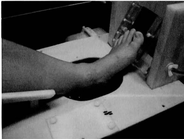
Figure 2.3 Leg-rest fixture for calcaneus bone positioning.
