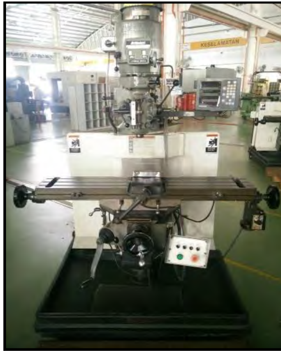
Figure 1.1: Bridgeport Vertical Milling Machine at Machine Shop at Block B of FKP
