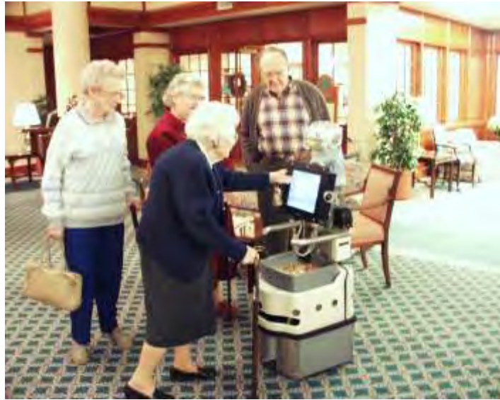
Figure 1.3: Pearl is a nursebot, which is also categorized as a social or service robot (Fong et al. , 2003)
