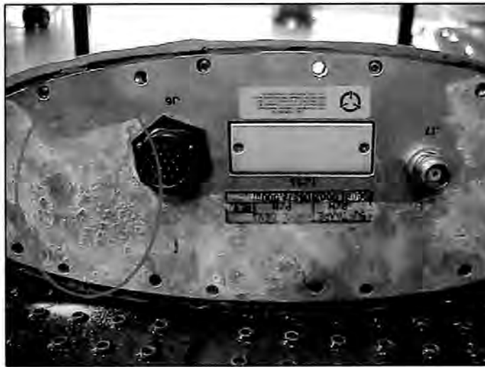
Figure 2.2 Salt causing corrosion to the antenna internal components because of a broken seal.
