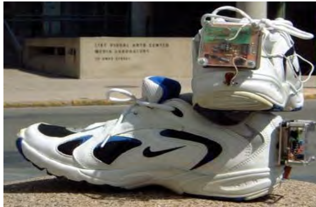
Figure 3 Example of design Piezoelectric Energy Harvesting Shoe
