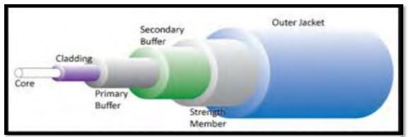
Figure 2.3:Basic structure of an optical fiber
