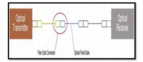
Figure 2.2: Simple Fiber Optic Link
