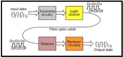
Figure 2.1 Basic fiber optic communication system
