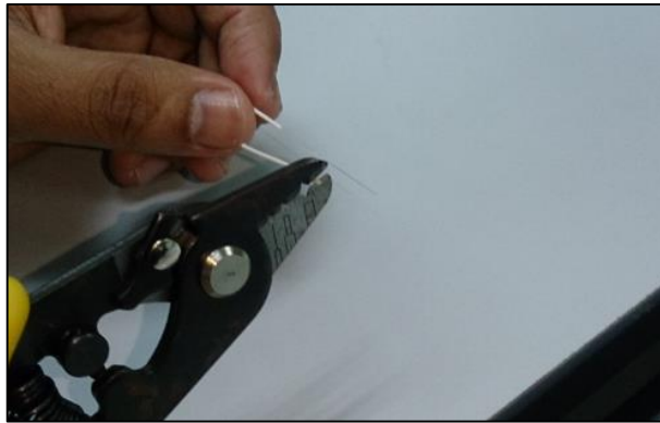
Figure 3.11: Stripping The Cladding of Fiber
