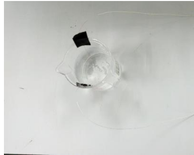
Figure 3.8: The position of fiber optic sensor inside the perfume during experiment
