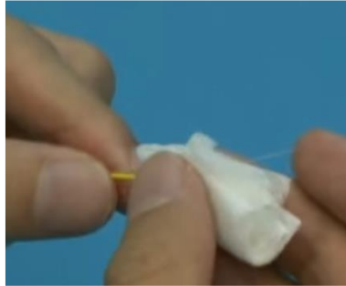
Figure 3.3: Dust removal process
