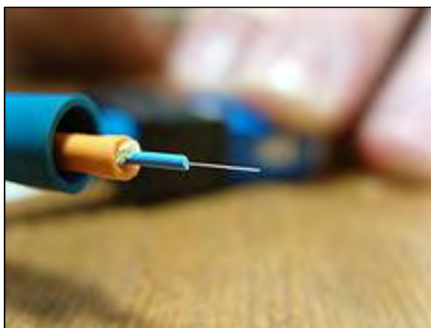
Figure 1.2: A stripped multi-mode fiber
