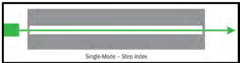
Figure 2.1 Single mode optical fiber propagation
