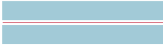
Figure 2.12: Light path in a single-mode fibre
