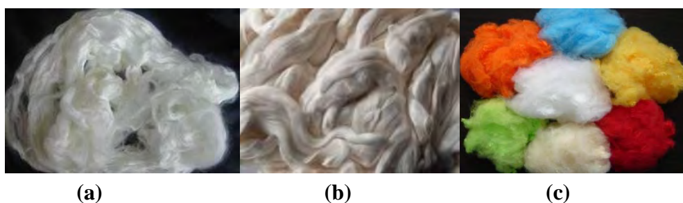
Figure 2.3: The example of synthetic fiber, (a) Acrylic (b) Rayon (c) Polyester
