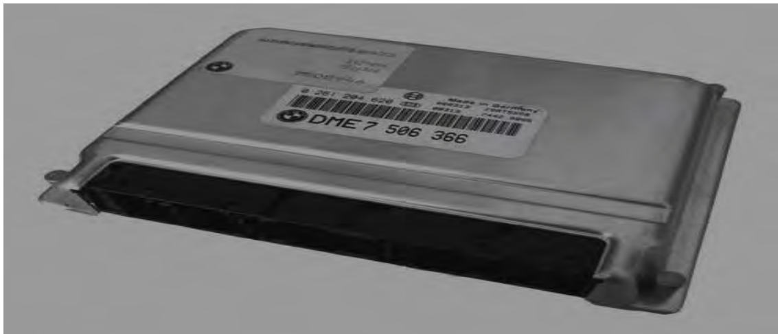
Figure 2.1 Bosch ECU of BMW X5 4.4i
