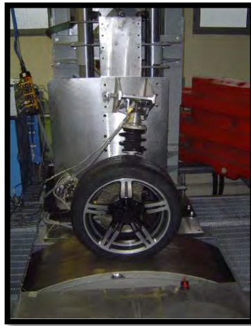
Figure 2.1: The RuotaVia test rig
