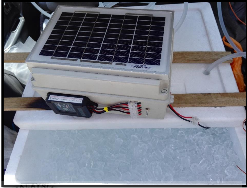
Figure 25 Picture of Mini Chiller and the Pump Connection to the Solar Panel.
