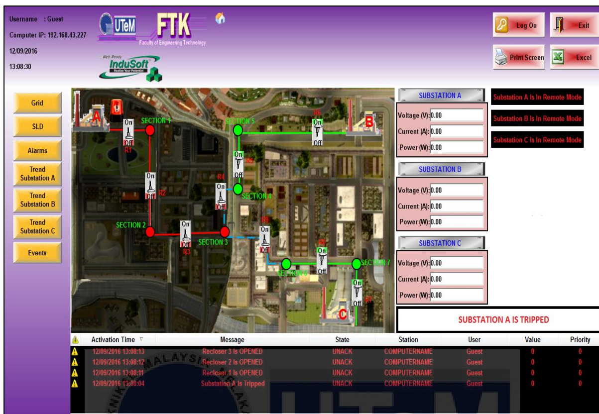
Figure 4.14: Fault occurred in sections supplied by Substation A.
