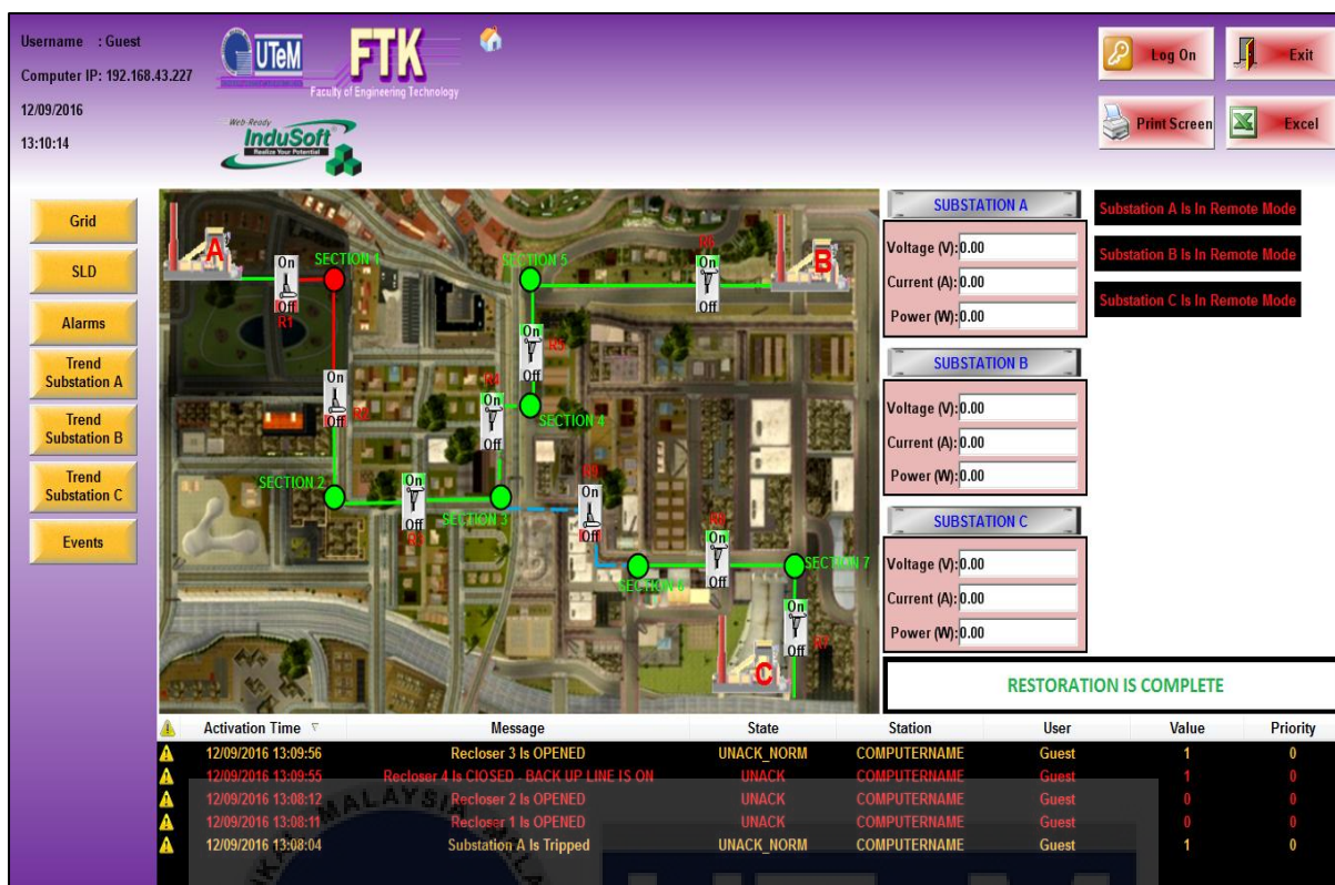
Figure 4.16: Section 2 is supplied by closing Recloser 3.
