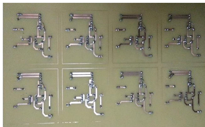
Figure 3.8 : MOSFET Driving Etching Circuit
