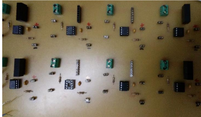
Figure 3.18 : MOSFET Driving Circuit
