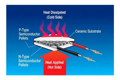
Figure 2.3: Generating Electricity from Thermoelectric Generator (TEG)
