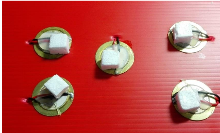
Figure 4.4.3: Latest project module PZT housing structure
