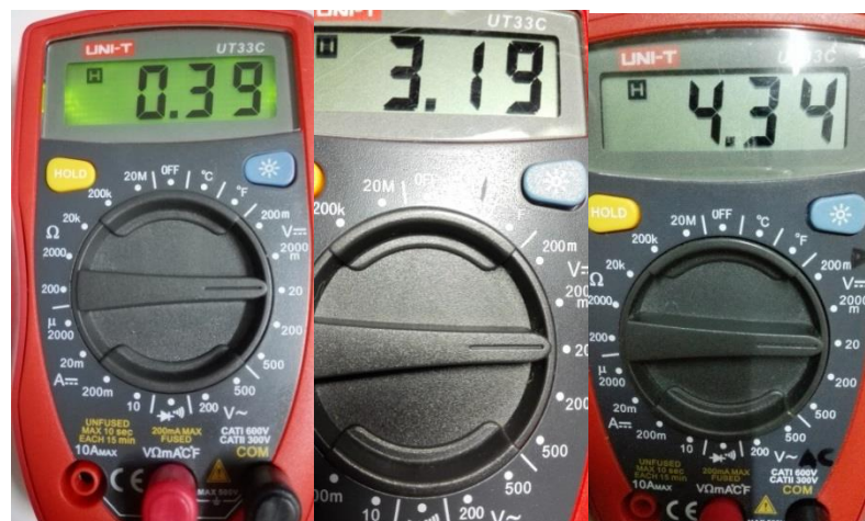
Figure 4.5.6: Multimeter shows the results of maximum DC Voltage obtained from PVDF
