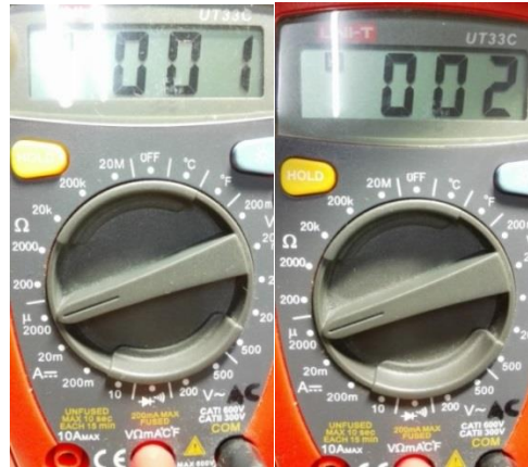
Figure 4.5.7: Multimeter shows the results of maximum DC Current obtained from PVDF
