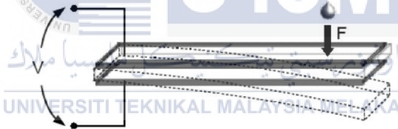
Figure 2.2.1: A raindrop hits the PVDF piezoelectric
