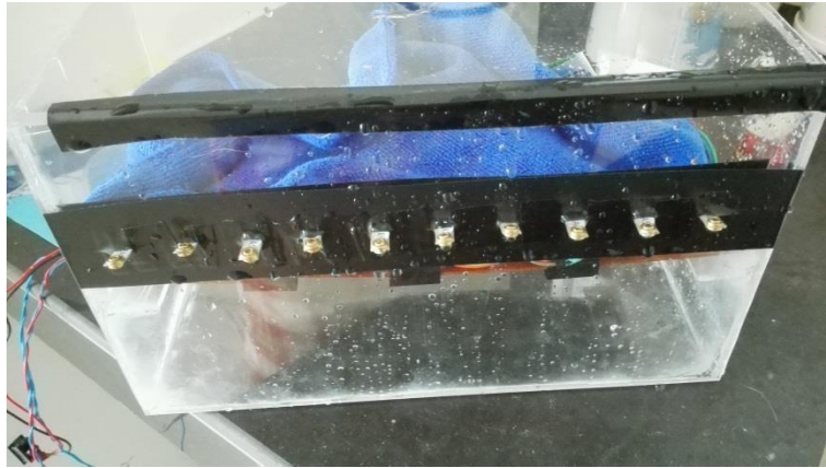
Figure 4.4.1: Latest project module PVDF housing structure
