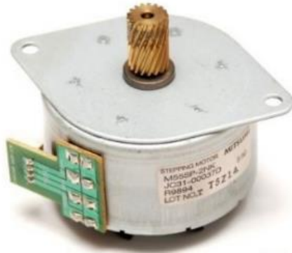
Figure 3.4 A stepping motor M55S-2NK with the label.
