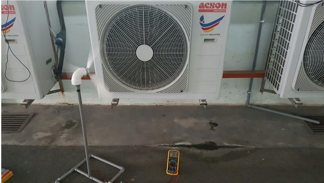
Figure 3.18 Process of data measurement for outdoor air conditioning unit.
