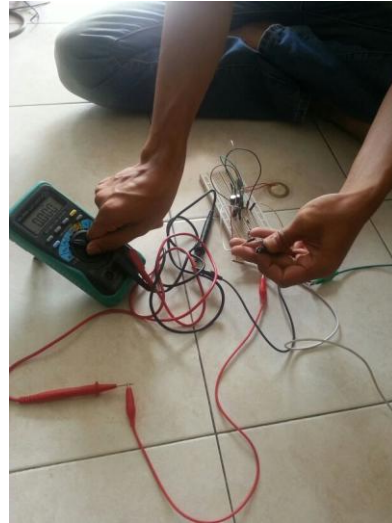
Figure 4.5.1: Tab the probe of multimeter at the series condition
