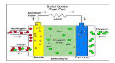
Figure 2.1: Basic principle of fuel cell
