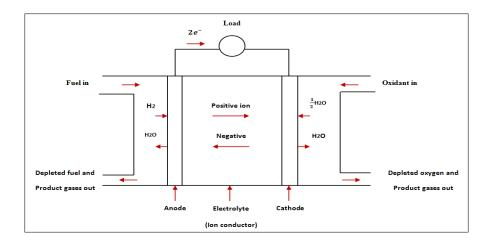
Figure 1.1: Basic working concept of fuel cell
