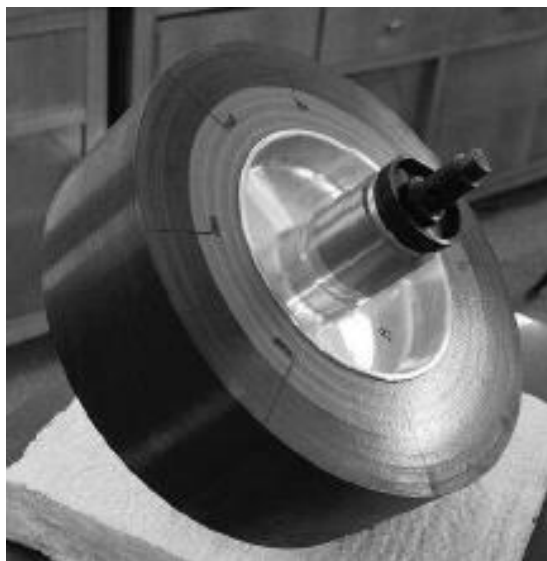
Figure 2.1: Example of flywheel rotor (Source: Bai, Zhang, and Wang 2012)
