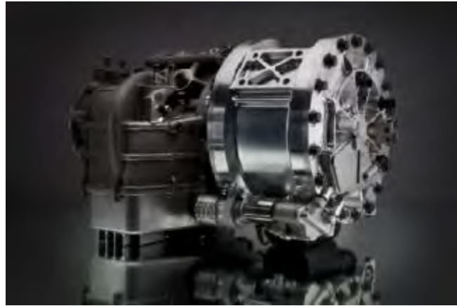
Figure 1-3: Jaguar hybrid car flywheel(Cibulka 2009)
