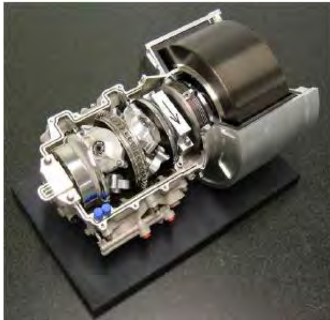
Figure 1-2: Formula 1 Flywheel Hybrid System 2009 season.(Cibulka 2009)
