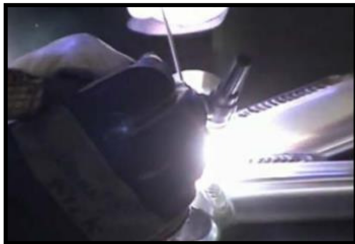
Figure 2.1: TIG welding the head tube of an aluminium bicycle frame.
