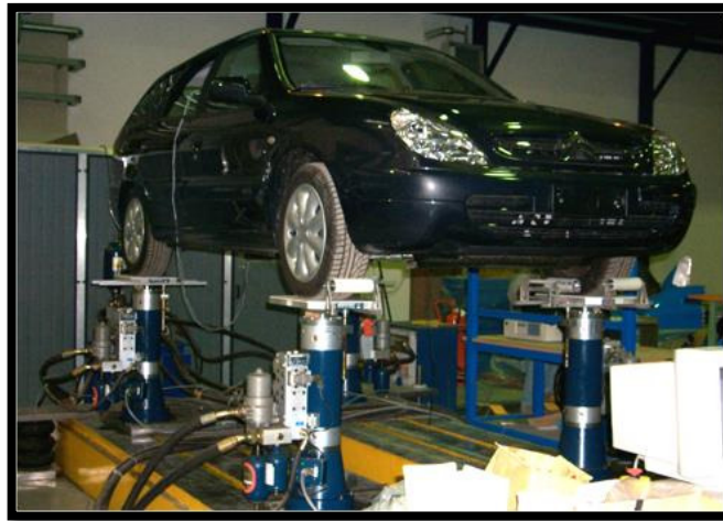
Figure 2.1: Vehicle on four poster (Vetturi et al., 2007)
