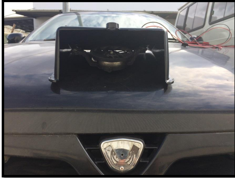
Figure 3.27: Wind turbine with air scoop
