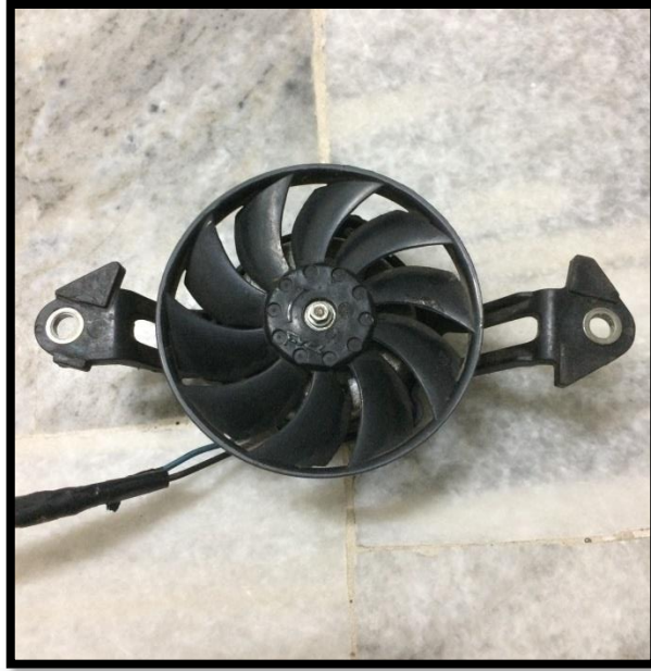
Figure 3.24: Turbine with diameter 93mm
