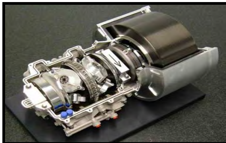
Figure 1.3: Flybrid System Formula One Flywheel Engine
